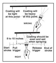
For best results, use 3 to 6 psi fluid pressure. Higher than 6 psi fluid pressure may be required for heavy-bodied materials. Low fluid pressures will produce a narrower than normal spray pattern. Generally use 30-35 psi air at gun inlet. Unusually heavy, difficult to atomize fluids may require up to 50 psi air at gun inlet.
